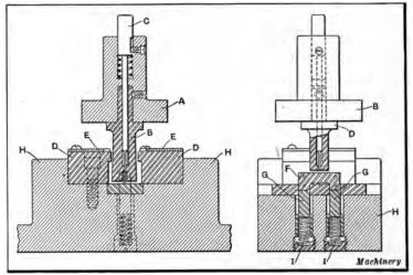
Fig. 6. Sectional Views of Staple Bending Die
